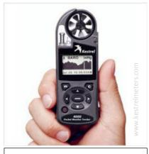
Handheld Kestrel sensor to measure thermal comfort
